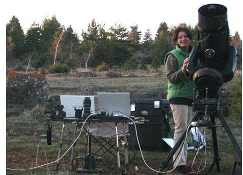
Fig. 3: Imaging set-up in France, Celestron 11", getting ready to take flat-fields.
