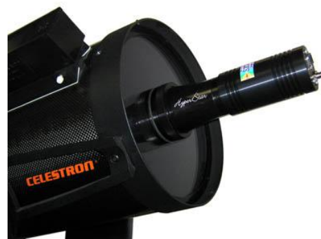
Fig 2: Celestron SCT with Hyperstar lens & Starlight Xpress CCD attached. Credit: Starizona-web
